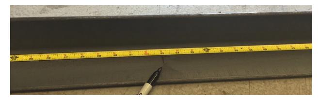
Using the supplied welder's jig, place the center notch cut-out on top of the line you made with the Sharpie marker or paint pen. Grab the Pivot Mounting Assemblies and "tack" (DO NOT PERMANENTLY WELD) into place at each end of the jig (make sure center notch stays on the top of the line marked on the center of the angle iron.
