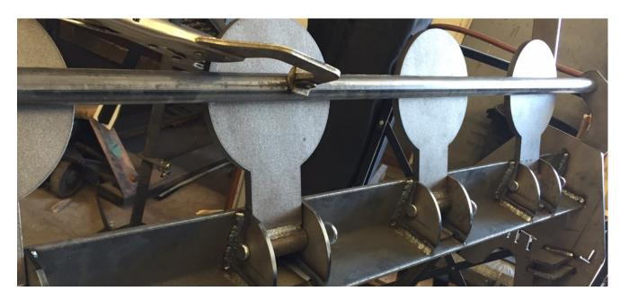
At this point, you are ready to weld in the 1" round bar permanently. For this portion, you only need a few good "tacks" to permanently weld in the bar. Two 1/2" beads on each side of the bar will provide a permanent hold. See picture below.
