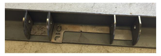
Use the jig to evenly space assemblies along the angle iron. Make sure all the paddle retaining holes are closest to the back edge (see photo). Now weld into place
