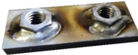
Once all 10 of the nut plates are completely welded, it’s time to weld the nut plates on to the arms of the Texas Star. We highly suggest cutting the arms to about 20” in total length, but you can certainly make them little bit longer if you’d like. The arms **MUST** be made from 1.5” x .25” angle iron
